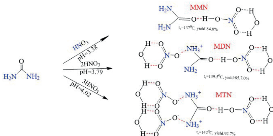
Scheme I. Reaction scheme for the synthesis of urea nitrates.
